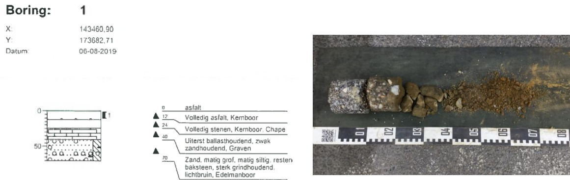
Figuur 6: Resultaten kernboring (ABO nv, 2019)
