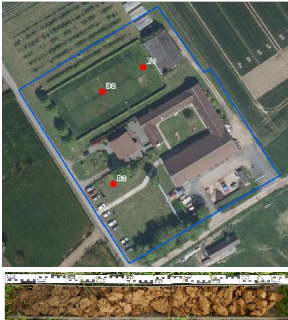
Figuur 18: Referentieboorkolom 1 [onder]; inplantingsplan controleboringen [© Hembyse]
