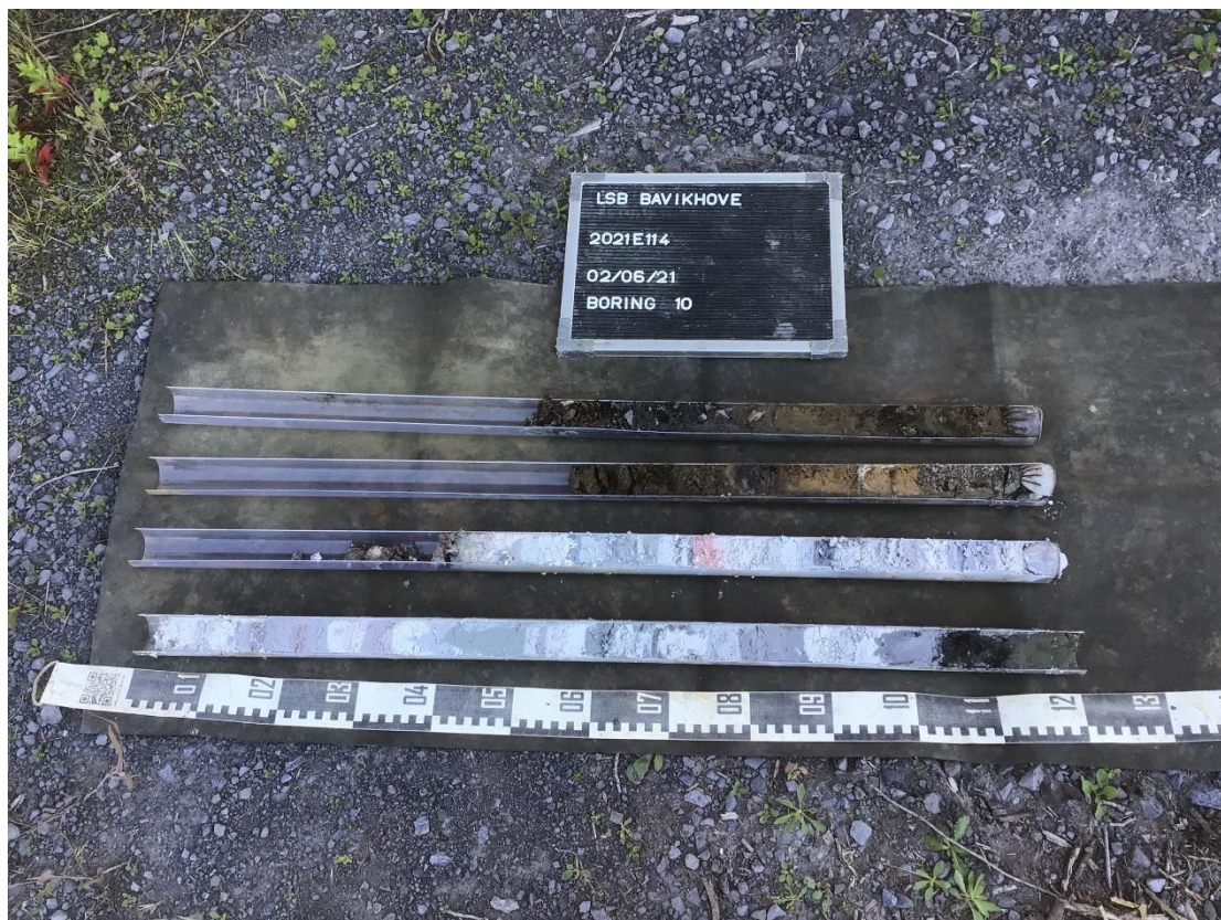
Figuur 18: Boring 10. © Geosonda 2021
