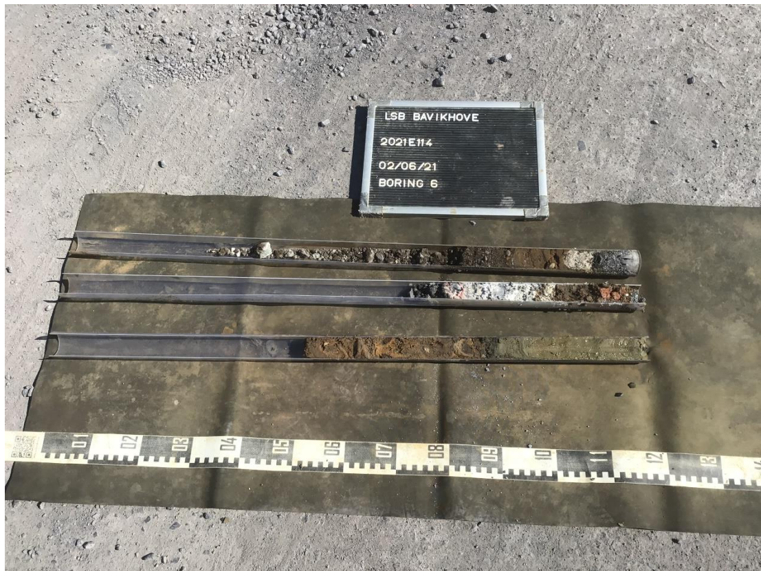
Figuur 14: Boring 6. © Geosonda 2021
