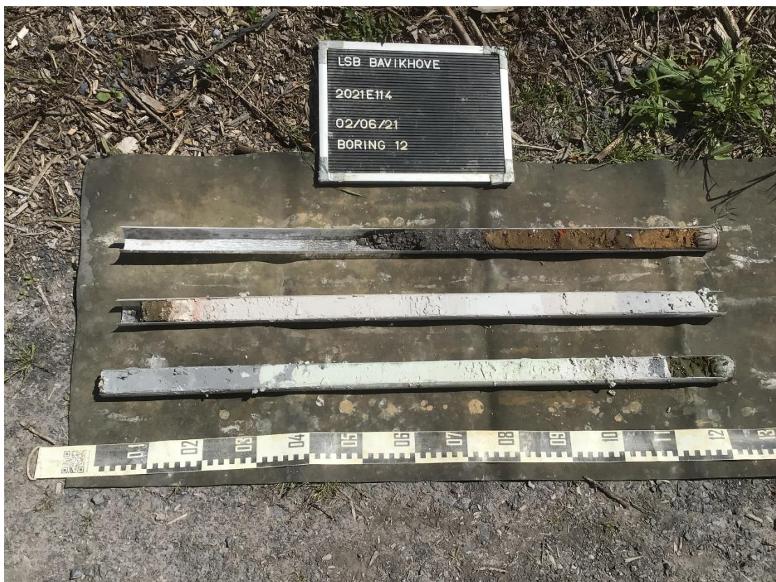
Figuur 20: Boring 12. © Geosonda 2021
