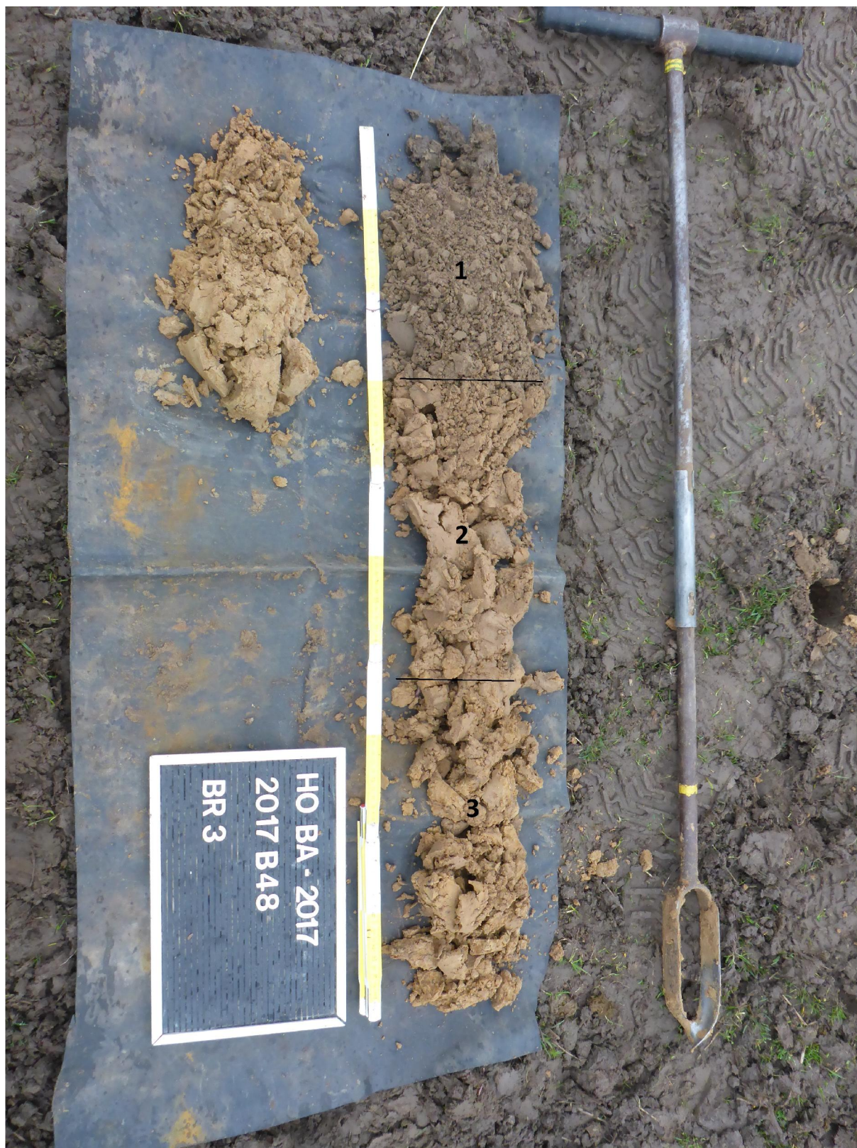
Fig. 24: Profiel van controleboring 3 (bron: © GATE).
