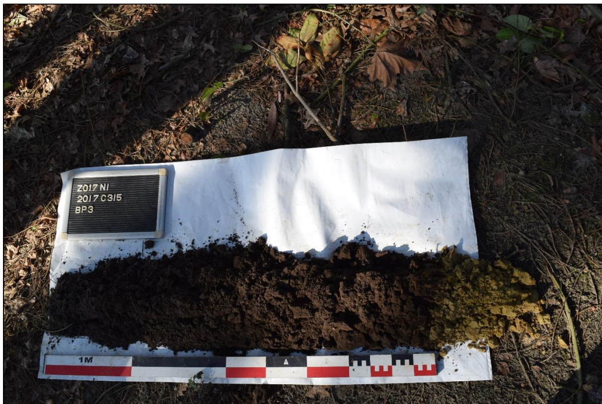
Afb. 30: BP 3 met horizonten ophoging – Ap1 – Ap2 – Bh – Cg (Bron: Aron bvba, dd. 23/03/2017, 2017C315)
