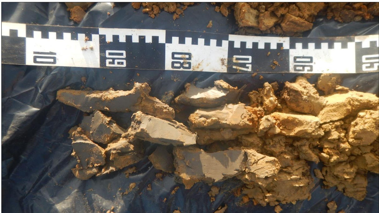
Foto 13: Boring 3, detail kleiafzettingen (©BAAC).
