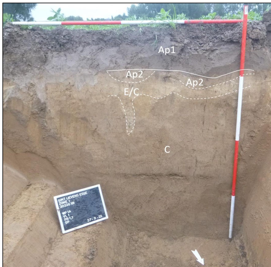
Figuur 7: Putwandprofiel 1.1 in zone 1 (ABO nv 2022)
